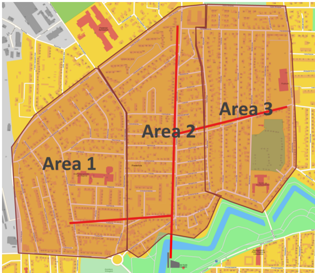
Figure 4: Placement of the main pipes in the district heating area
